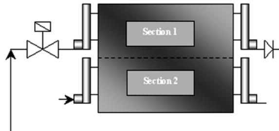
Both sections of the coil are normally operational in mechanical cooling mode only. When the free cooling mode is activated, i.e. when outdoor air T2 is lower than  $(T1 - \Delta T)^{\circ}\text{C}$ , and mechanical cooling operation is requested at the same time (integration), section 1 is cut off and ventilation can be forced at maximum rate, though maintaining an excellent control of condensation pressure.
