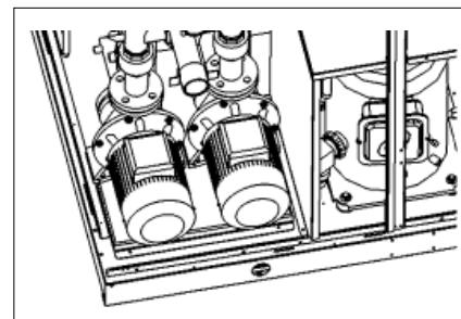
In the case of installation on roofs or intermediate storeys, the unit, pipes and air intake/outlet ducts must be insulated from walls and ceilings by placing rigid rubber joints in between and using supports that are not rigidly anchored to the walls.
