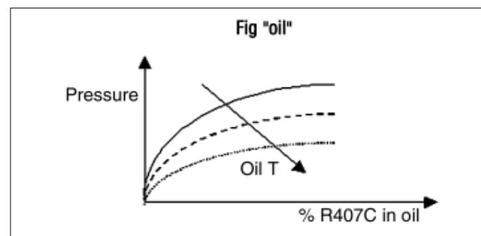
The use of heating elements is particularly important especially at first start-up. In this connection it is recommended that they are switched on at least 12 hours before the compressors are started.
